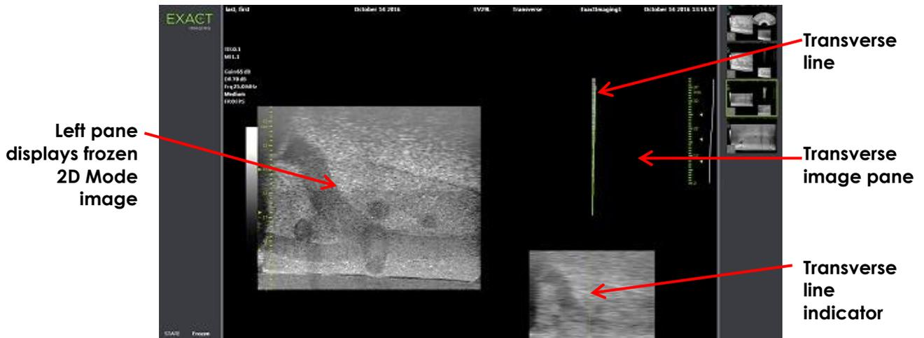
Figure 45: Transverse Mode Before Transverse Image Construction
