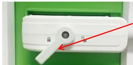
Figure 21: Transducer Connector Orientation
