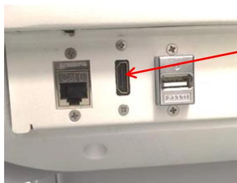
**Figure 11: Second monitor output (HDMI) Connector**
