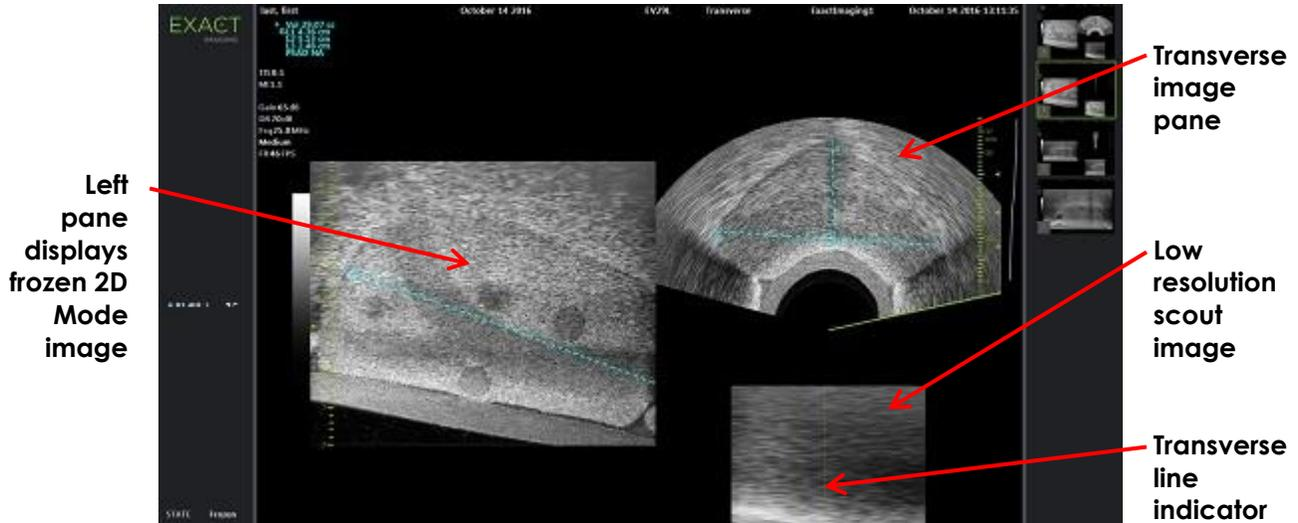
**Figure 46: Transverse Mode After Transverse Image Construction**
