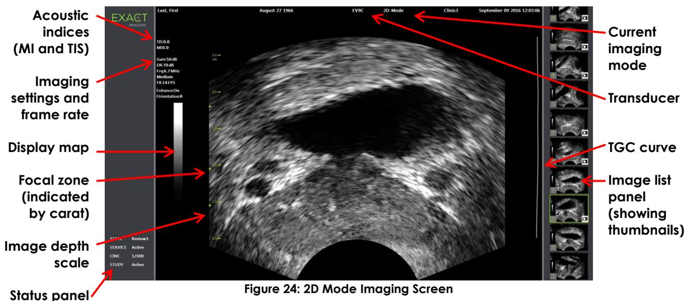
Figure 24: 2D Mode Imaging Screen
