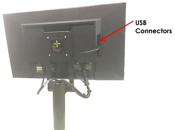
**Figure 8: USB Connectors on the Rear of the Monitor (available in some ExactVu system configurations)**
