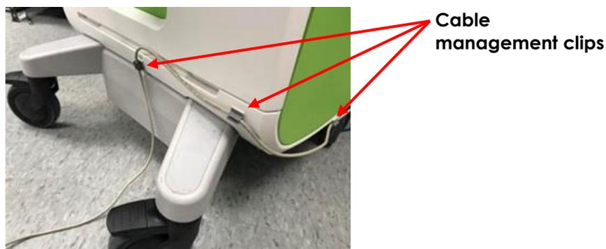
**Figure 4: Foot Pedal Cable Management**
