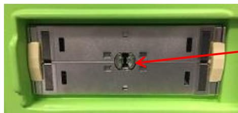
Figure 20: Lock Notch on the Transducer Connector Slot
