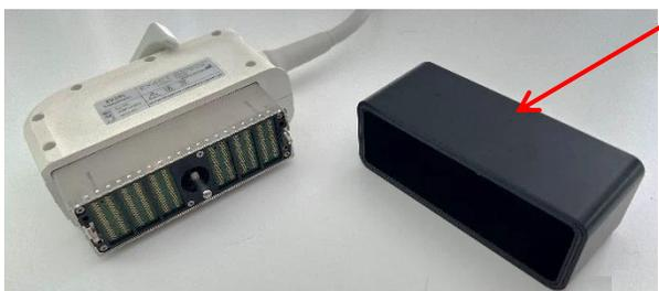
Lockable transducer connector cover (i.e., a large-sized cover)
