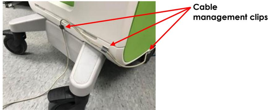
**Figure 4: Foot Pedal Cable Management**
