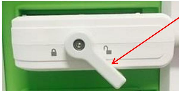
Transducer connector lock knob (in the unlocked position)
