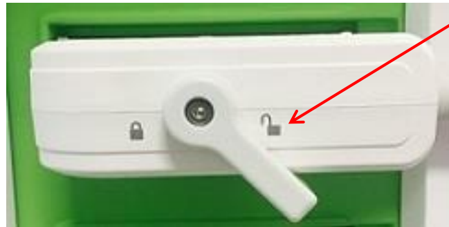
Figure 9: Unlocked Transducer Connector Lock Knob
