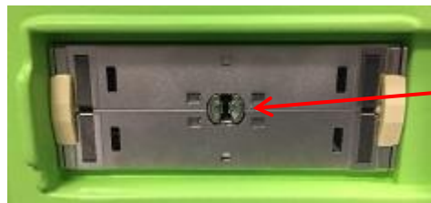
Figure 7: Lock Notch on the Transducer Connector Slot
