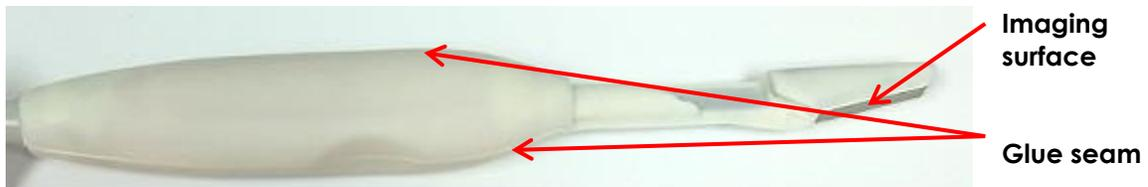
Figure 33: EV29L Transducer
